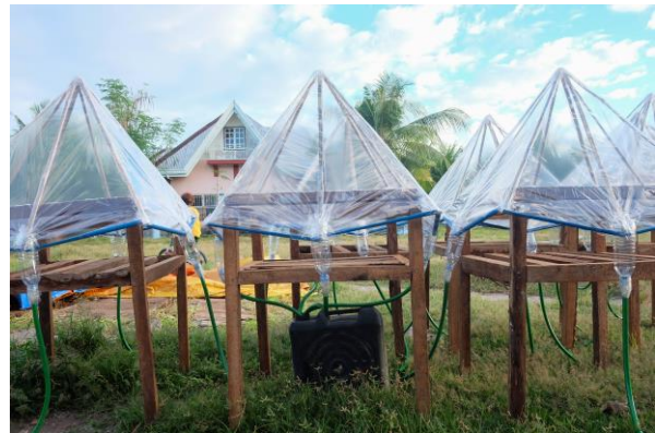
The desalinators which are able to produce 3 litres of water a day
